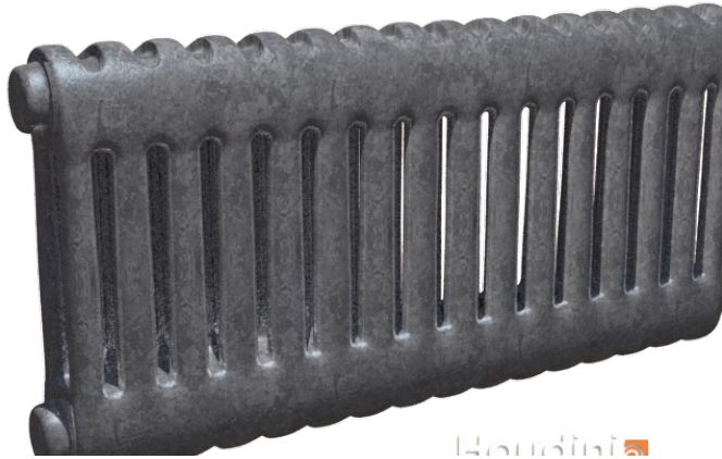
a1: Subdivided model of a heating radiator with parameters for size, radii and divisions.
